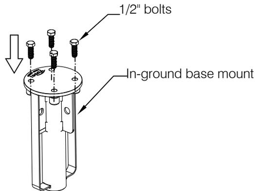
Step3. Pour concrete and insert in-ground base mount thru center of the concrete slab.
