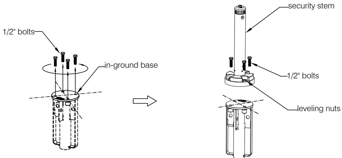
Step 6. The SECURITY STEM may not be exactly 90 degree to create a level canopy. Use the LEVELING BUBBLE as a guide to better adjust the level of the SECURITY STEM. Adjustments should be made with the canopy as a reference point, not the SECURITY STEM. Once the canopy is level, securely tighten all 4 screws (1/2" - 13) with 3/4" wrench.
