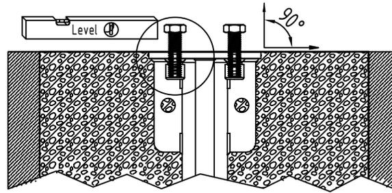
Step 5. Once concrete is cured remove 1/2" mounting bolts (4-places) . Place the security stem on the in-ground base mount and reinsert the 4 mounting bolts into the leveling nuts. Screw the mounting bolts into the in-ground base mount, NOTE: do not tighten the bolts completely .
